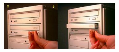
This procedure cannot be repeated without cycling the DVD-ROMs (computer's) power. After the media is removed and the loading tray is closed, the tray will not reopen without first turning the power ON/OFF.
